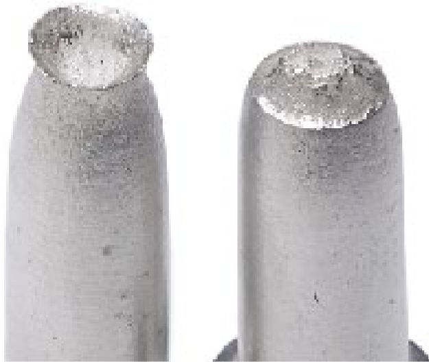
cup-and-cone fracture - moderately ductile
