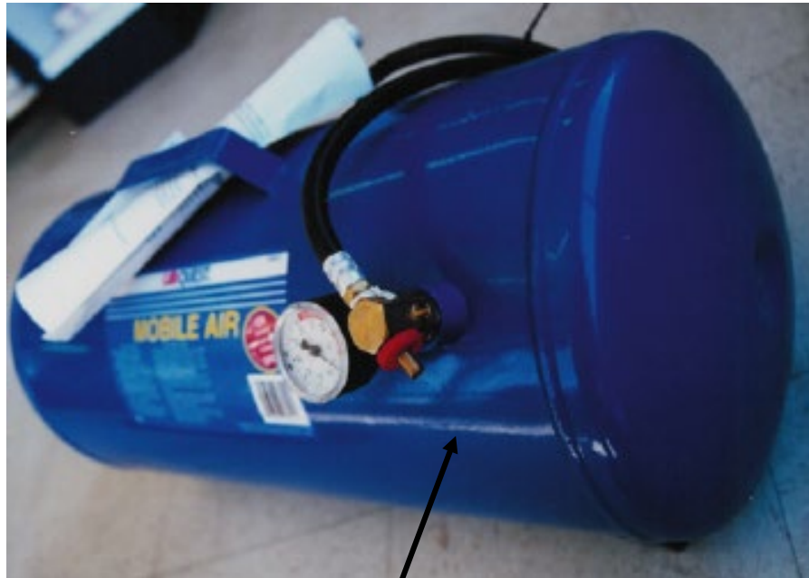
Pressurized tank (photo courtesy P.M. Anderson)
